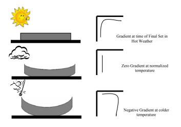
Figure 2: Effect of changing temperature gradients on amount of slab/construction curl
