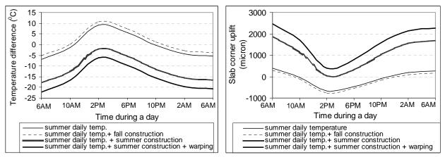
Figure 15: Temperature difference between top and bottom of slab during a typical summer day and slab corner uplifts during a typical summer day under the four climate loading cases (Hansen et al). Data from I-94 project (12.5 in. thick pavement).
