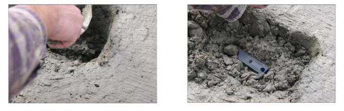
Figure 10: Scooping out of fresh concrete and placement of tags (University of Michigan, Ann Arbor)
