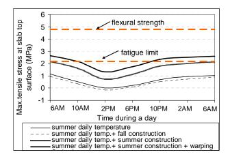
Figure 16: Tensile stresses at slab top surface under combined climate and truck loadings
