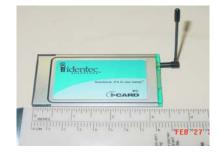
Figure: The i-Q32T tag/transponder and the PCMCIA card transceiver. (Wake Inc.)
