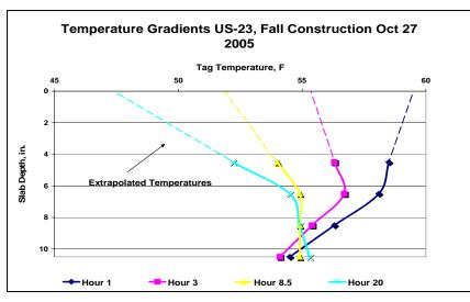
**Figure 14b:** Difference of temperature and the gradient in slab up to time of final set. Temperature data provided by Tim Stallard, MDOT (Hansen et al)
