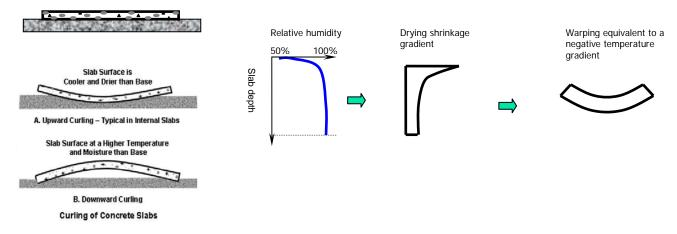
Figure 7: Slab curling phenomena due to temperature gradients and due to rapid drying shrinkage (NRMCA CIP 19 and U of Michigan)
