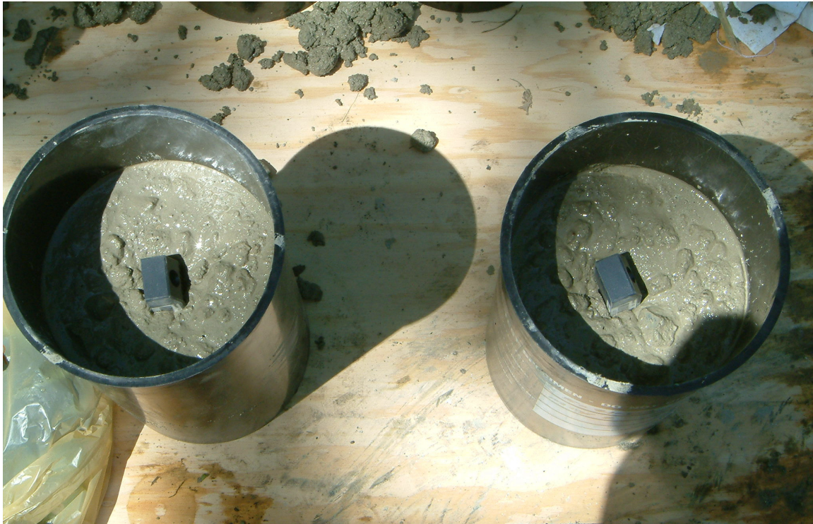
Figure 5 IQ8T Tags placed in cylinders
