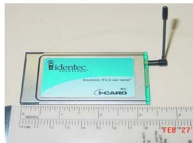
**Figure:** The i-Q32T tag/transponder and the PCMCIA card transceiver. (Wake Inc.)
