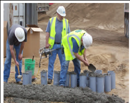
Construction crew making Test Cylinders
